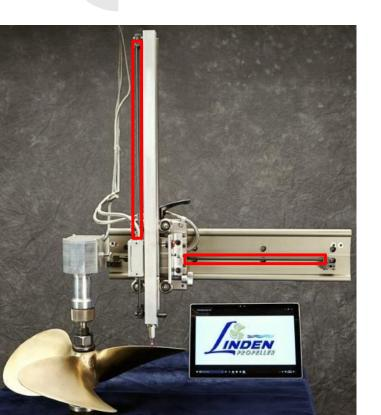
Project Name: Laser Scan Readings for Propeller Measurement
